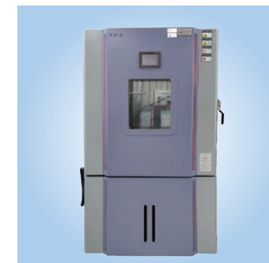
High and low temperature environmental test chamber
