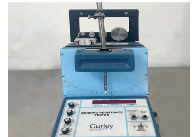
Filter paper stiffness tester
