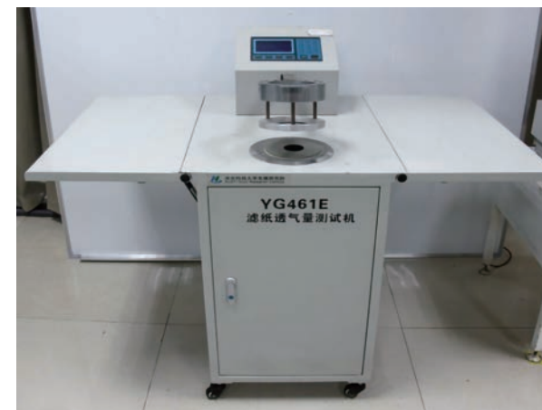
Filter paper air permeability tester
