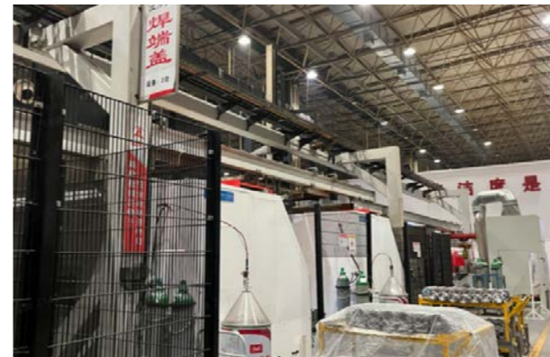
| Welding cylinder base | Automatic pairing, high welding accuracy
