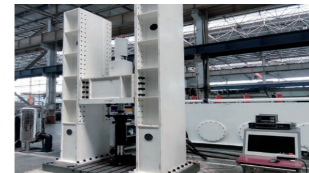
Pneumatic suspension test bench
