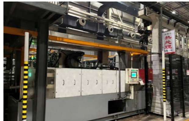
| Surface quenching | High surface hardness, long lifespan
